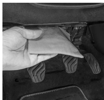
Figure 2: Clean the installation site
